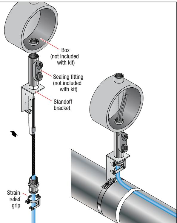
**Input Power Splice** (for power connection to two lengths of heater – additional kits required)
